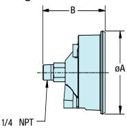
Gauges are important for monitoing the operating pressure or vacuum of the blower. Gauges should be positioned as close to the blower as possible.
