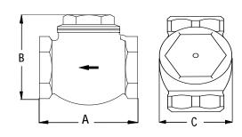
Swing check valves allow air to flow in one direction. These valves prevent backflow into the blower and are supplied in bronze or brass.
